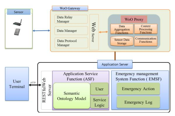
The WoO gateway is capable of communicating with sensor nodes through various communication mechanisms and protocols. It also has the capability to relay environmental data to the WoO proxy in active and passive mode. In active mode sensors shall push data to the gateway, and in passive mode
