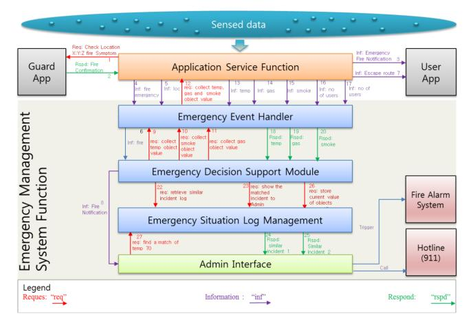
The ESLM module receives the temperature, gas and smoke object value as a query and returns the similar incident data as output to the admin interface. The manager is the person authorized to manage the emergency situations by accessing the admin interface. He can customize the actions according to the necessity and retrieve any required data from ESLM. ViOs are related with each other through the semantic ontology model and can provide the current object value in RDF format.
