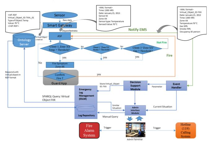
Figure 14. Sequence diagram for emergency fire management system.
