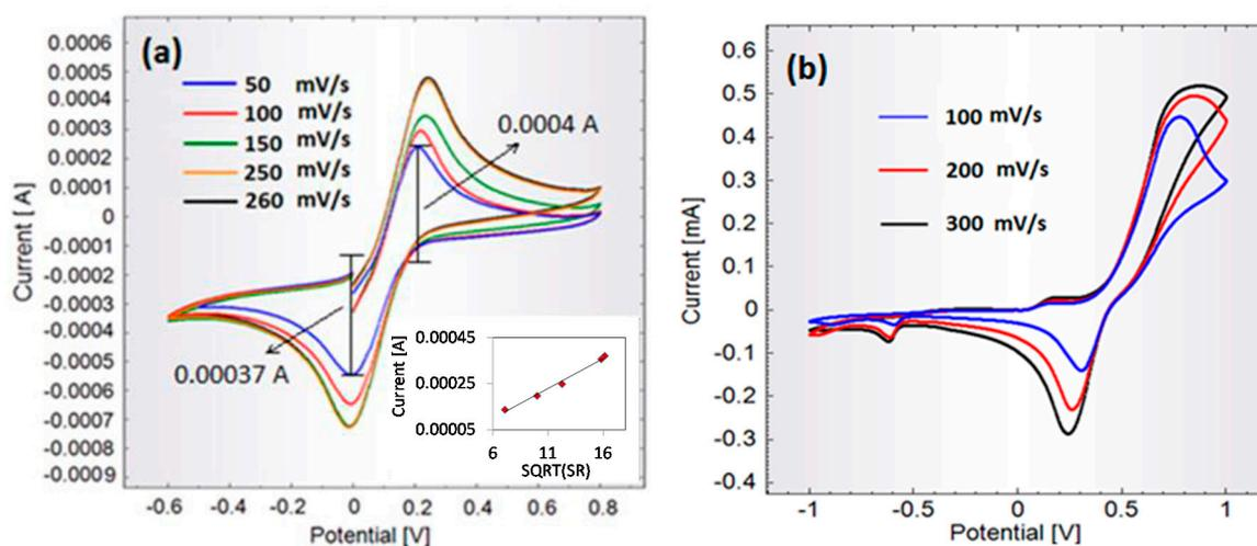
It is seen that the numeric ratio between the current peaks is almost unity (example in figure: 0.0004 A/0.00037 A) and that the peak potentials are independent of the sweep rate. The inset in Figure 2a
