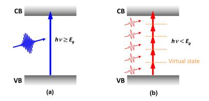
Figure 3. Laser processing of transparent material using (a) long pulses and (b) ultrashort pulses.
