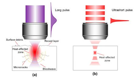
Figure 3 schematically illustrates the interaction of long and ultrashort laser pulses with a transparent material. Compared with conventional laser fabrication techniques that use continuous wave (CW) lasers or lasers with nanosecond pulses, femtosecond laser processing has several distinct advantages:
