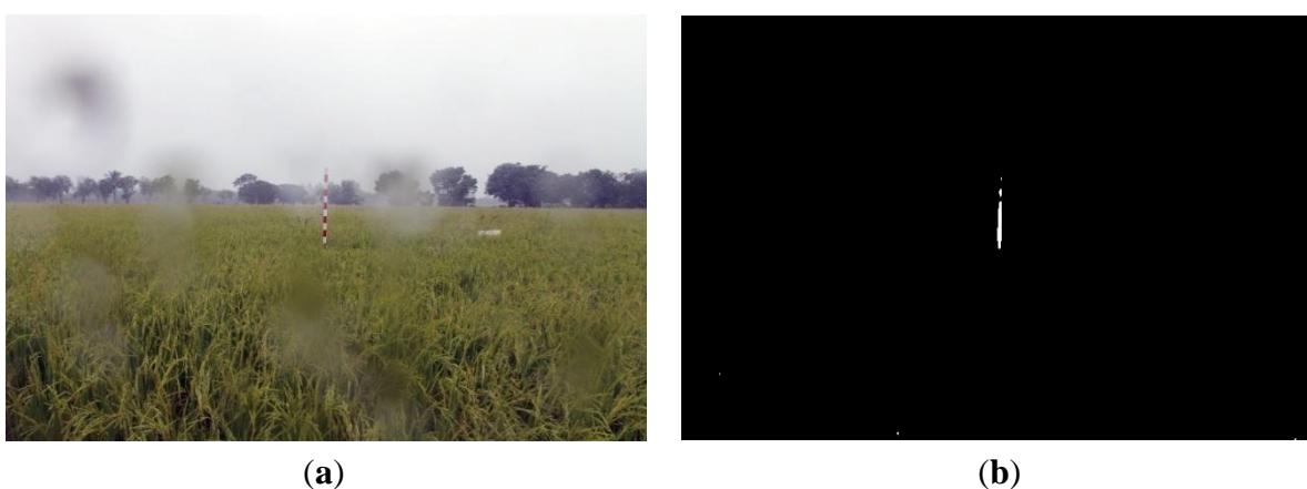
Figure 22. Comparison between (a) RGB and (b) resultant binary images using proposed method with excess green feature in case of rainfall on 25 July 2012.
