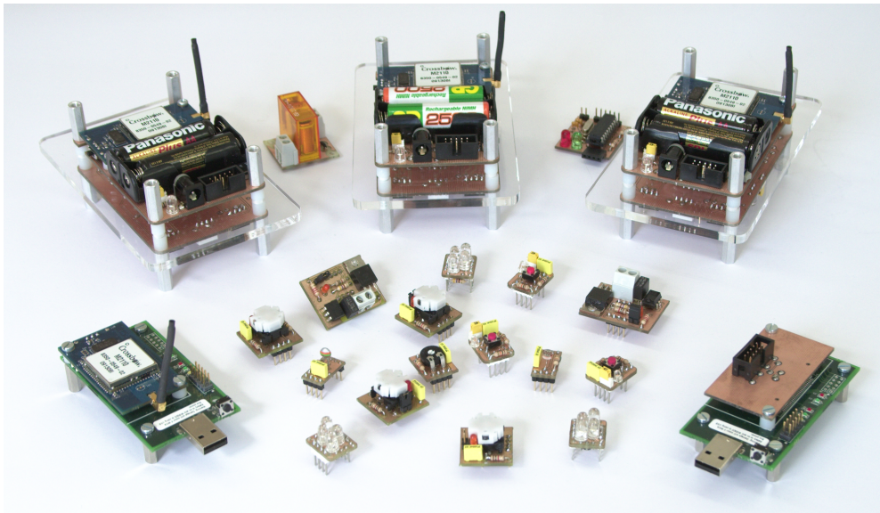
Figure 9. Motebox demonstration kit using UVPN.
