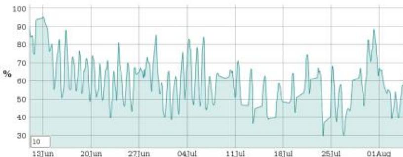
**Figure 11.** Masonry crack: 55 days log.
