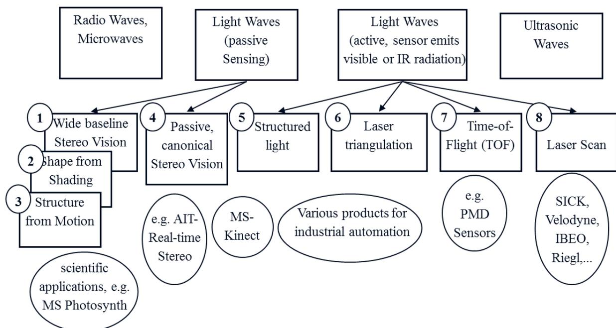
Methods 4, 7 and variants of 5 provide such a single-shot capability. Due to resolution limitations and relatively high costs, TOF sensors (7) appear less suitable for leg edema quantification. Thus, methods based on real-time stereo vision, structured light or a combination of those seems to be suitable for leg edema quantification. Up to now, such methods have not been evaluated for leg edema detection.
