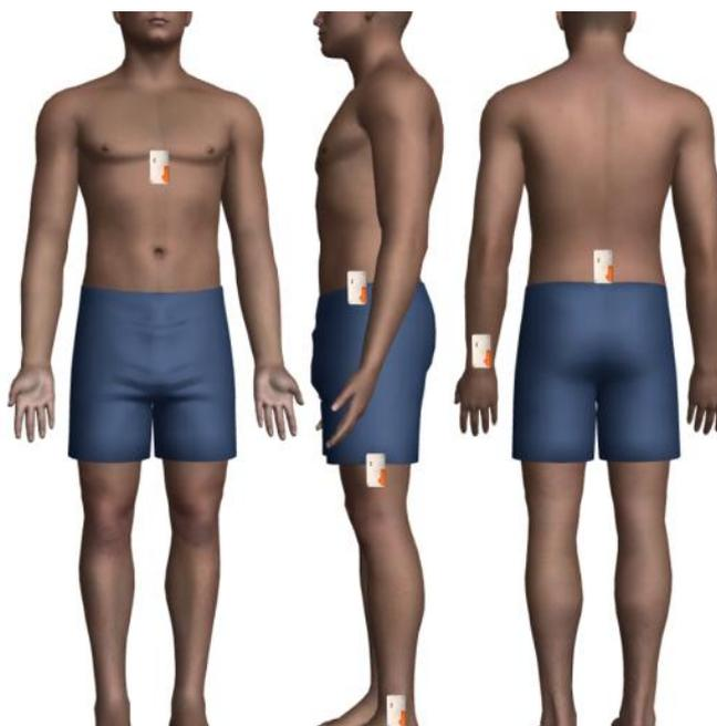
Acceleration data was collected using six Shimmer wireless sensor platforms (Shimmer 2R, Realtime Technologies, Dublin, Ireland). These tri-axial accelerometers had a range of  $\pm 6$  g and sampled data at 51.2 Hz. This sampling frequency is sufficient to capture most everyday activities (~20 Hz) [3]. Bodily acceleration amplitude can range up to  $\pm 12$  g. Nonetheless, the literature suggests
