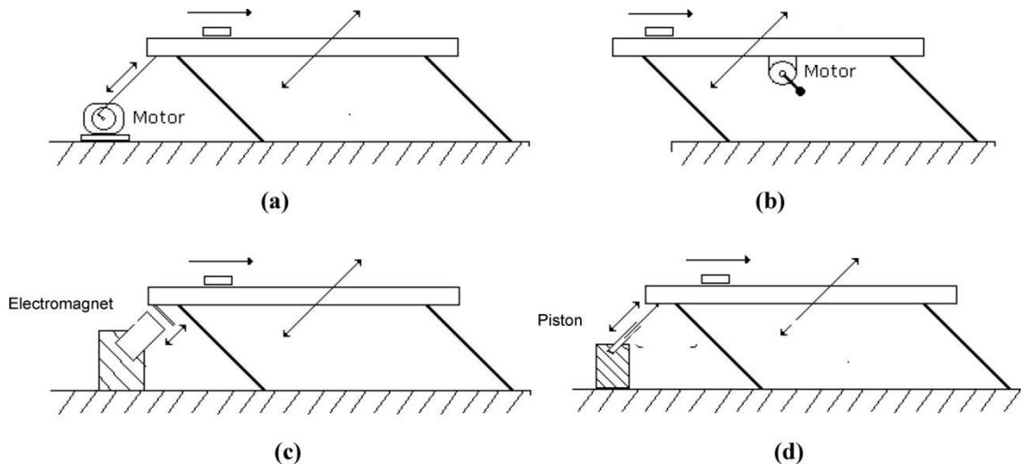
This paper addresses an alternative excitation mechanism for vibratory feeders, which is based on the use of piezoelectric actuators for motion generation. Variants of this concept have been the subject of some patents [3,4] and some models are commercially available [5,6]. More recently, a study comprising the dynamic modeling and experimental assessment of a piezoelectric vibration feeder based on parallel bimorph beams has been presented [7].
