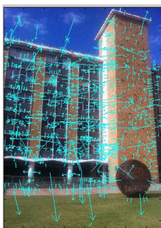
Figure 9. Reference feature database generated for the candidate image space: 13182 features from 20 reference images in the image space.
