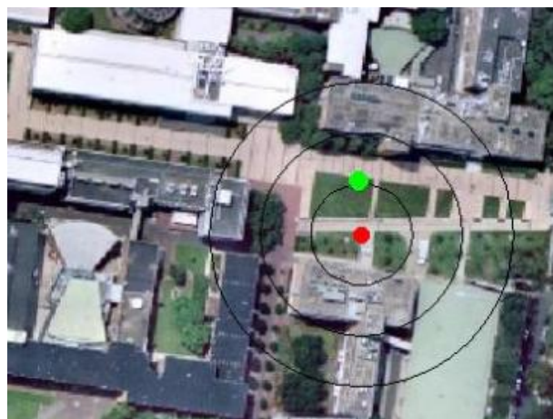
Figure 15. Positioning result for the query image shown with green dot. The red dot indicates the location determined by the GPS, with the black circles show the process to enlarge the search space (1–3 times of its horizontal precision).
