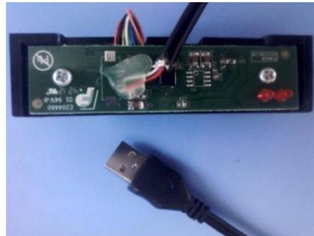
The principle is basically the same as the line-controlling ones. The only difference is that an USB converter is added between the chip and the USB interface, as depicted in Figure 13. The additional USB converter makes it easier to test the performance of the sensor chip. It can obtain the card information from the terminal through the USB interface directly.
