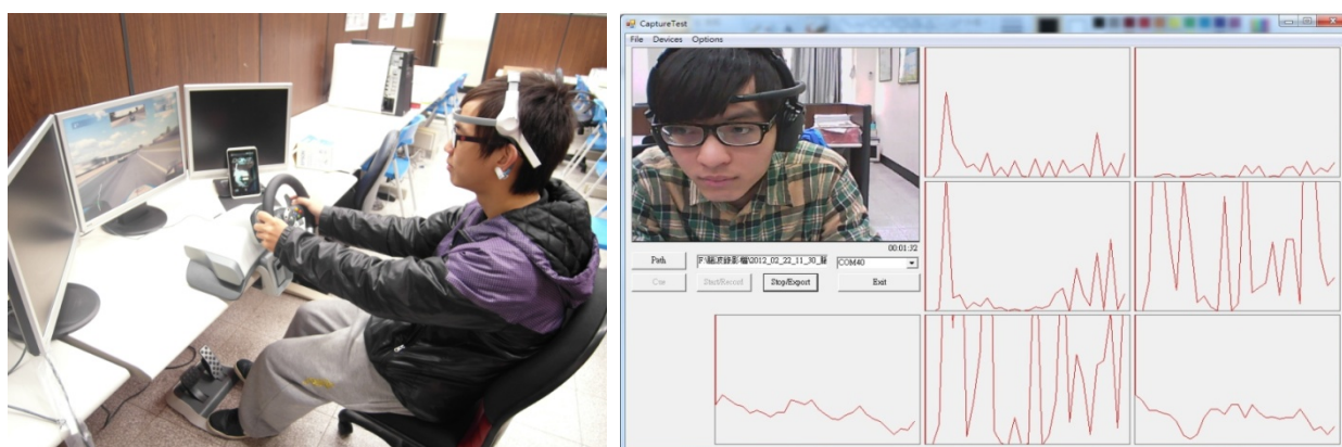
Figure 7. A driving simulation system for the collection of driver's brainwaves.
