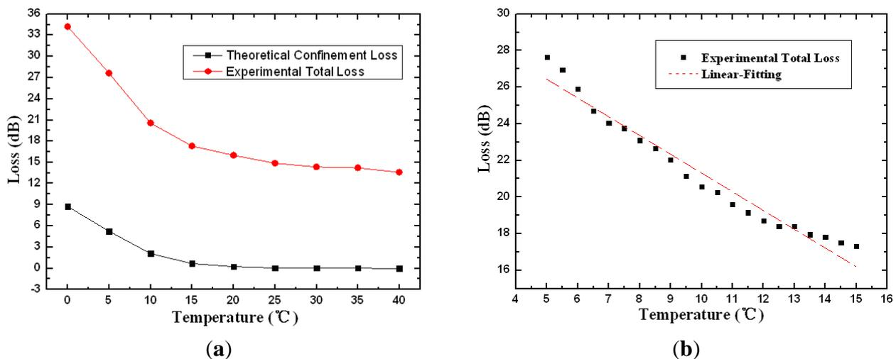
**Figure 6.** Theoretical and experimental loss (a) and linear fitting curves of the experimental loss (b) as functions of temperature with pure chloroform.
