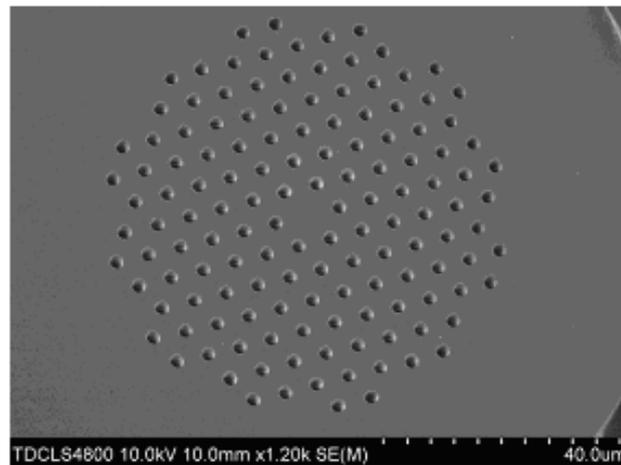
Liquids such as ethanol, toluene and chloroform present high temperature-dependent optical sensitivity. PCFs infiltrated with these materials are susceptible to external temperature variations. The refractive index of the background material  $\text{SiO}_2$  is calculated according to the Sellmeier equation [19]. In the liquids, the temperature behavior of the refractive index is assumed as a linear approximate expression:
