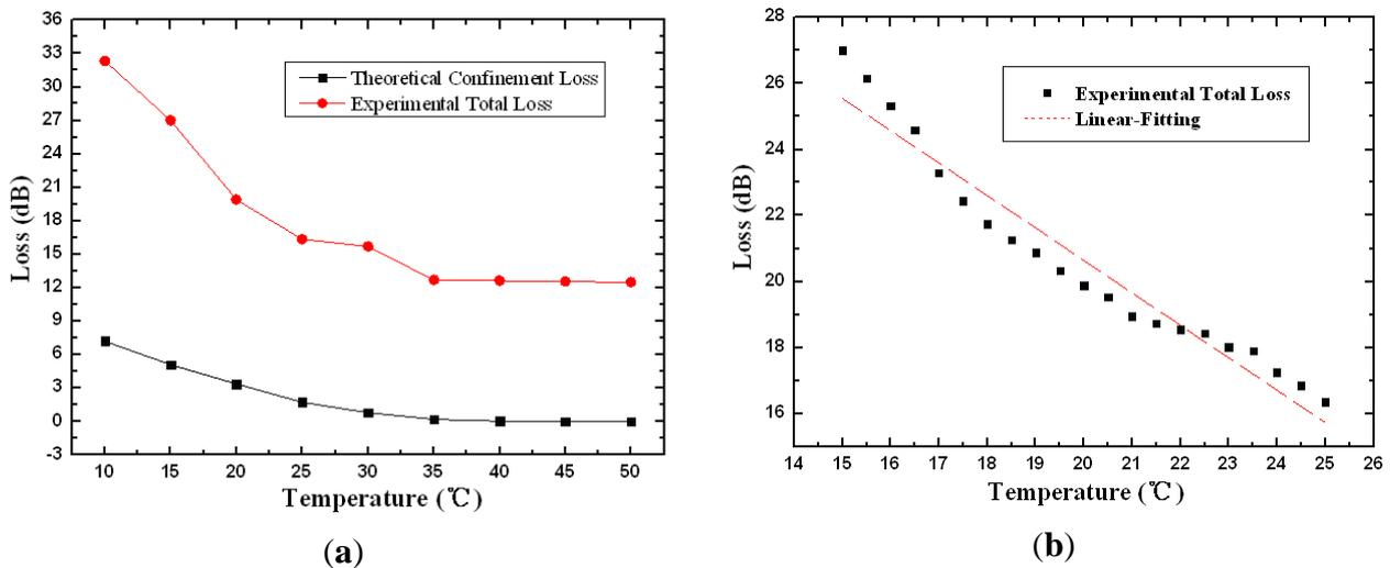
The similar simulated and experimental results have been shown in Figure 6(a), while the linear fitting curve have been plotted in Figure 6(b) with pure chloroform filled into the air holes. The attenuation decreases from 32.3 to 12.5 dB within the temperature from 10 to 25 °C. The linear fitting expression is given in the temperature sensitive range from 15 to 25 °C:
