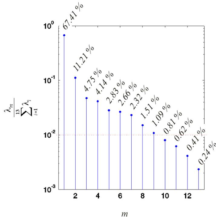
**Figure 7.** PCA coefficients of the test deviations from the desired swing motion. For test observations 1, 2, 3, and 5, at least one coefficient exceeds the acceptable range, indicating improper motion in the associated swings.
