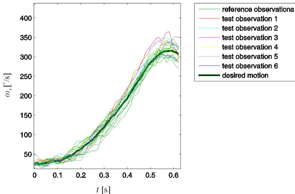
Note that not all improper swing motions could be detected by directly comparing the test and reference observations. Test observations 1, 2, and 3 in Figure 4 could eventually be detected. However, test observations 4 and 5, although referring to improperly performed swings, could not be distinguished from the reference observations.
