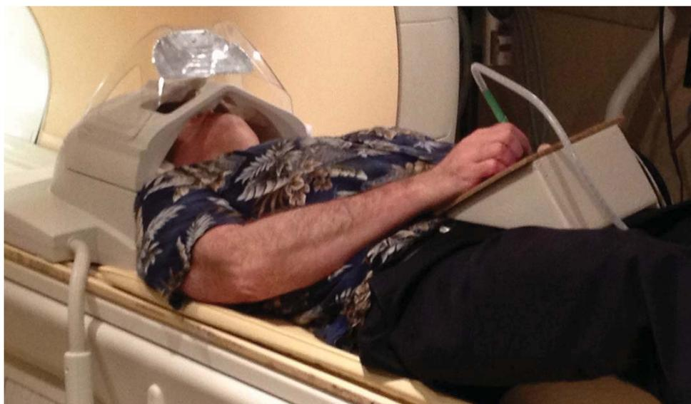
We tested the fMRI-compatible pen with two 11 year-old subjects while they were performing writing tasks in a 3T scanner. Each task was presented in two 4-minute blocks to be used in an fMRI connectivity analysis preceded by a 6 second reminder instruction screen. Stimuli within each block were pseudo-randomly selected.
