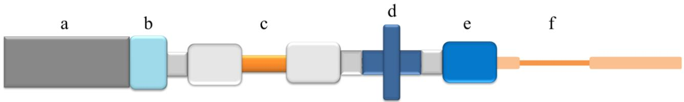
**Figure 11.** Schematic of the tool used for qualitative analysis of the optical transmission defects: (a) laser source; (b) collimator; (c) fiber cable; (d) fiber adapter; (e) fiber connector; (f) processed fiber; and (g) micro-stage.
