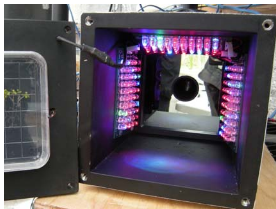
Figure 6. Grow lights boards and positioning within the TIS-III.
