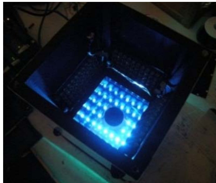
Figure 8. TIS-III excitation LEDs behind a band-pass filter.
