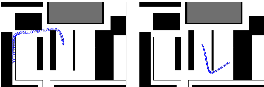
Figure 12. Two examples of optimal paths computed using AICO in a static environment.
