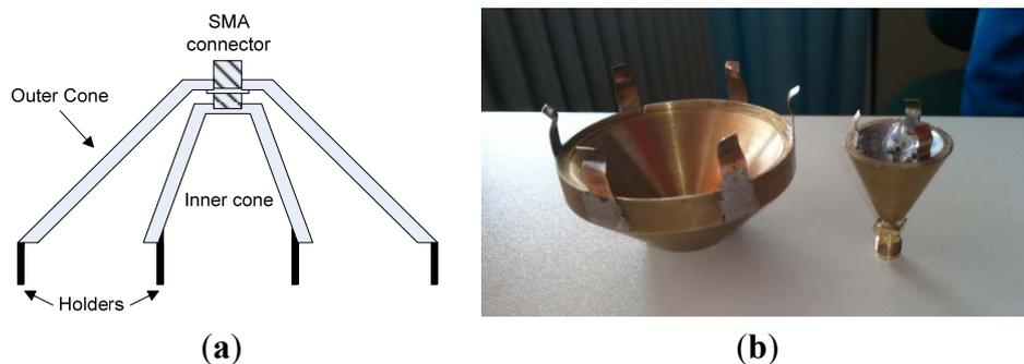
**Figure 3.** The proposed sensor (on the right) and its parts.
