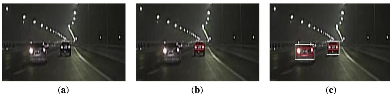
**Figure 10.** (a) A scene where a reflective light block is in the middle of a pair of taillights; (b) Using the global detection algorithm; (c) Using the proposed algorithm.
