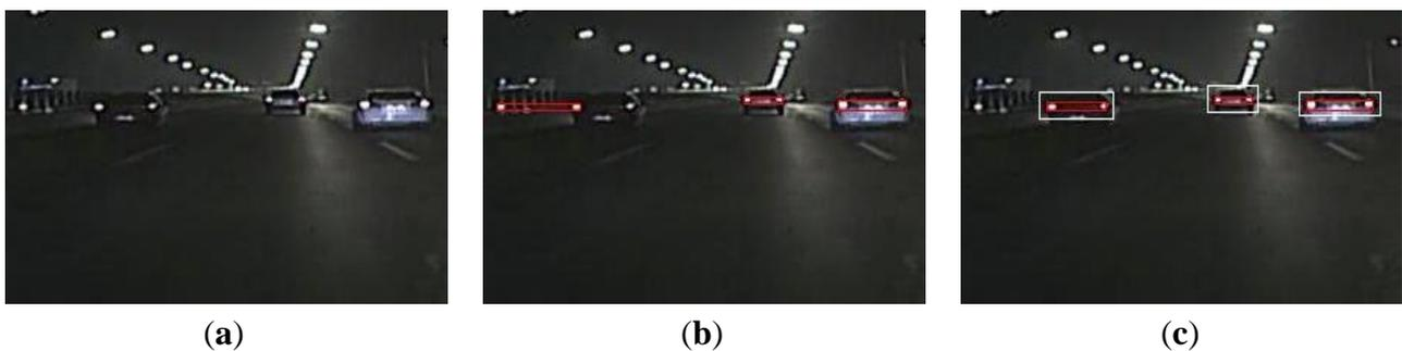
In comparison to the existing vehicle detection algorithms, another advantage of the proposed algorithm is the adaptive thresholds utilized in the rules of taillights extraction and pairing. The thresholds are adapted in real time according to the corresponding vehicle information in the previous frame. This mechanism could effectively reduce the false positive and false negative detections, as shown in the traffic scenes of Figures 9–11.
