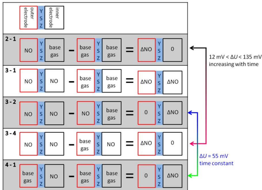
Whether or not the gas difference with “zero value” stems from NO at the same electrode ( $\Delta U_{3-2}$  with NO at the outer electrodes and  $\Delta U_{3-4}$  at the inner electrode, respectively) or base gas at the same electrodes ( $\Delta U_{2-1}$  with base gas at the inner electrodes and  $\Delta U_{4-1}$  at the outer electrodes, respectively), there are the same difference curves, *i.e.*,  $\Delta U_{2-1} = \Delta U_{3-4}$  and  $\Delta U_{3-2} = \Delta U_{4-1}$ .
