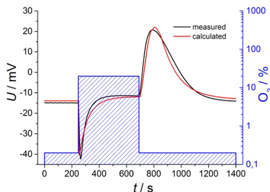
The curves are in very good accordance regarding amplitude and shape, so it is possible to describe the sensor voltage in detail by this simple calculation. This exemplary description includes Nernstian equation considering temperature difference between both electrodes, oxygen dependent thermovoltage and various time constants for gas diffusion, but only in a first order approach.
