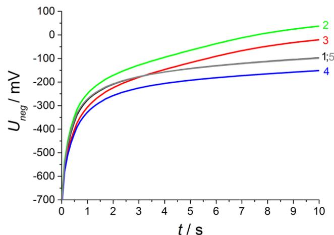
After turning off the NO dosing (phase 4), NO is only present at the inner (reference) electrode. This leads to a concentration difference with opposite sign compared to phase 2. The discharge voltage is at a higher level compared to phase 3, but the discharge is markedly faster as in phase 2 with opposite NO gradient. With increasing diffusion time, the discharge curve goes back to the base gas curve of phase 1 and only a small discrepancy is visible at the end of the diffusion time (phase 5).
