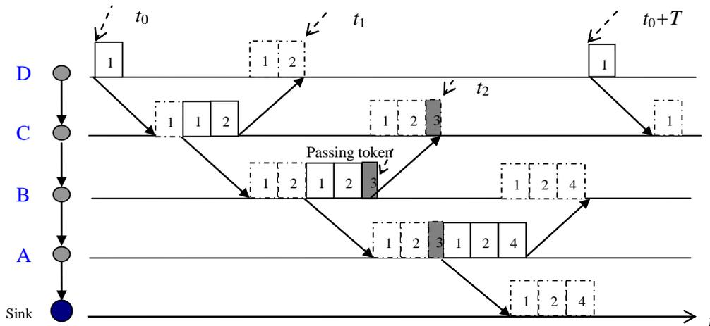
In the initialization phase, the sink assigns a pseudo-random binary spreading sequence to each established path in the network. It is assumed that the spreading sequence is orthogonal or quasi-orthogonal. In general, since the number of the established paths is much less than the number of nodes, the length of the spreading code used in POCA is much shorter than that of TOCA or ROCA.
