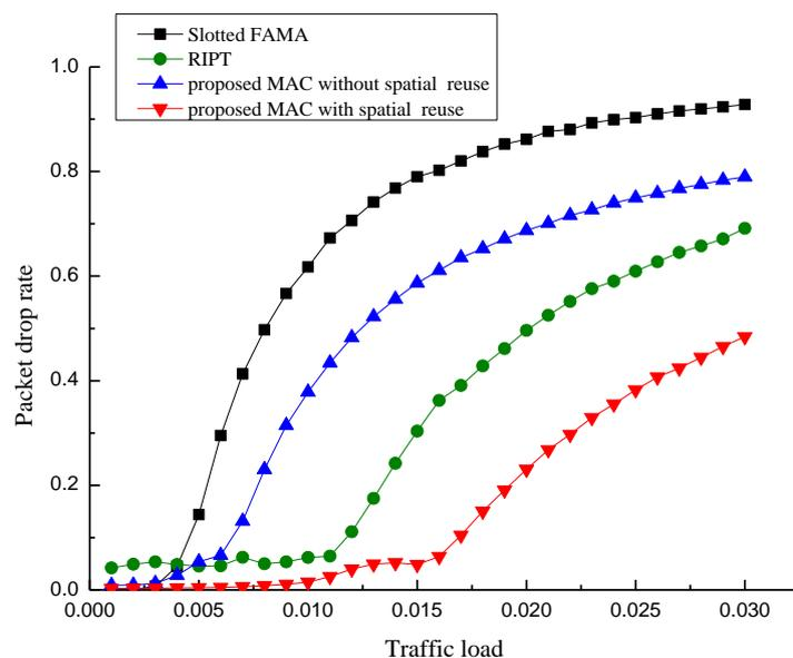
However, the packet drop rate of the proposed protocol without spatial reuse is larger than that of RIPT when the traffic load is larger than 0.05 packet/s. The reason is that the proposed protocol without spatial reuse uses too much time to forward the packets when long spreading sequences are
