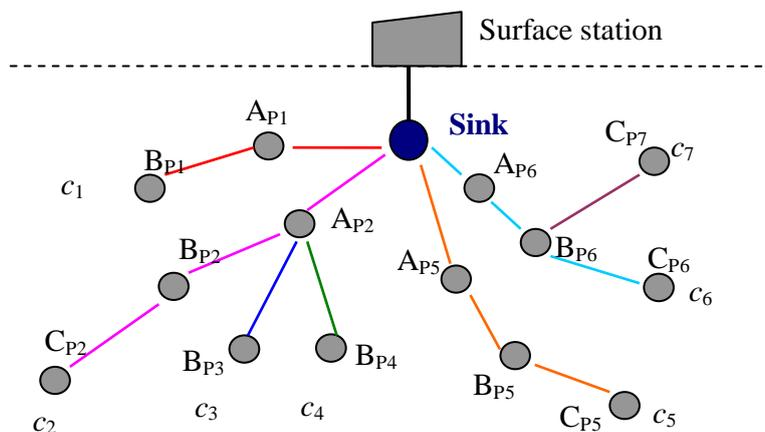
In the initial phase, the sink generates and sends spreading sequences to its neighbor nodes according to the number of established paths in the network. When  $A_{P1}$  received its spreading sequence ( $c_1$ ) from the sink, it transfers  $c_1$  to  $B_{P1}$ . The sink sends three spreading sequences ( $c_2, c_3, c_4$ )
