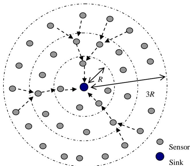
Let the maximum transmission range of sensor nodes be  $R$  km, the sensor nodes are uniformly deployed with the average density of  $\rho$ , and data packets in each node arrive in a Poisson process with the arrival rate  $\lambda$ .
