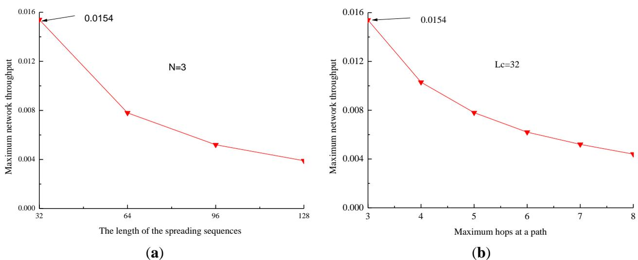
From Figure 8a, we observe that the maximum network throughput decreases quickly when the length of the spreading sequences increases. The reason is that the length of the data being transmitted increases quickly as the length of the spreading sequences increases, and the efficiency of the channel
