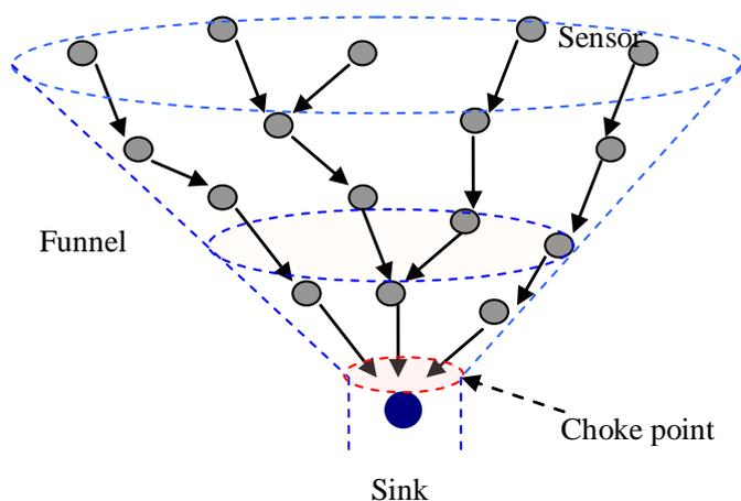
As shown in Figure 3, the sensor nodes are randomly deployed in a circular area. When the distance from the sink to the network edge is larger than the maximum transmission range of sensor nodes, the sensor nodes near the sink should act as the intermediate nodes to forward the data from sensor nodes located far away from the sink.
