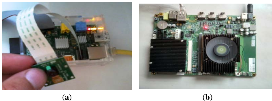
Figure 18. Scheme of the low-cost system. (a) Raspberry Pi and (b) A Carma-board.
