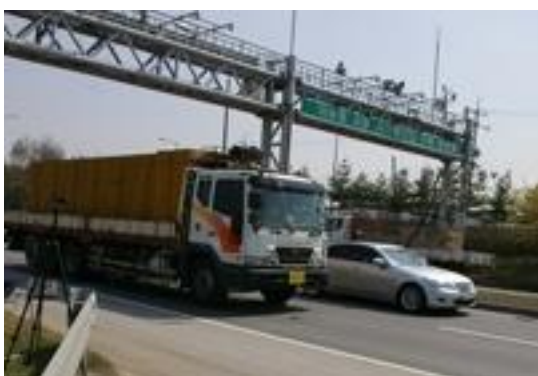
(c) Laser-based reference instrument and video recorder mounted over the road.
