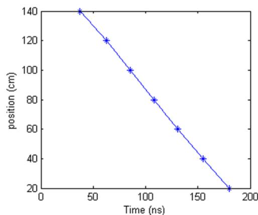
Figure 22 is the relationship between spike positions located by the oscilloscope from Figure 21 and the real deformation positions. It is a linear relationship. If choosing a straight line from the point at 20 cm to the point at 140 cm to fit the experiment results in Figure 22, the max location error is 1.6 cm. Using this method, the deformation points can be located by EHTSC.
