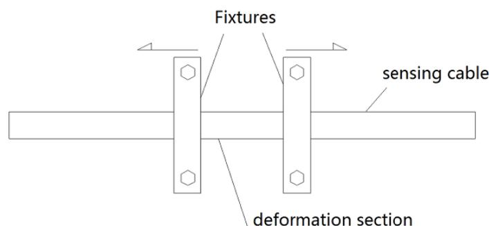
The length of the deformation section is 25.0 mm. Then the deformation section is stretched to 54.6 mm. Figure 16 shows the transient voltage in the initial state and the transient voltage when the cable is stretched. From the waveform in the red circle, we can see that there is a difference between the two waveforms. Compared with non-uniformity influence, the waveform difference caused by stretching is very small. To obtain deformation directly from the waveform is difficult.
