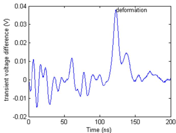
Figure 18 shows that there is a difference between two initial transient voltage waveforms. It means that the uncertainty of TDR device will affect the difference waveform whether deformation is happened.
