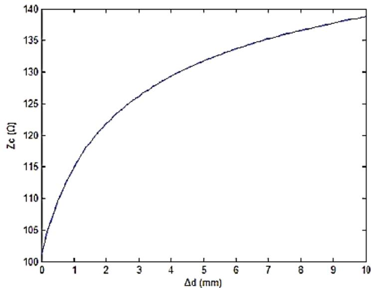
The relationship curve shows that EHTSC's impedance increases when the cable is stretched and the rate decreases when  $\Delta d$  increases. That means EHTSC can effectively detect the deformation in a certain range near  $\Delta d = 0$ .
