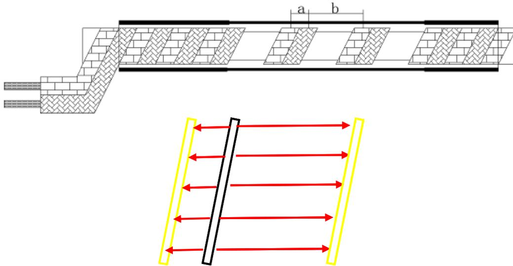
If the signal frequency is high enough, most of charge will be on the surface of the wires. According to the parallel wires capacitance calculation method, the distributed capacitance can be written as:
