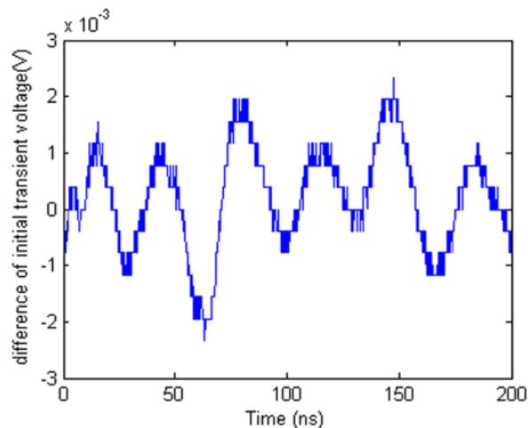
**Figure 19.** Change of transient voltage waveform with different deformation section lengths.
