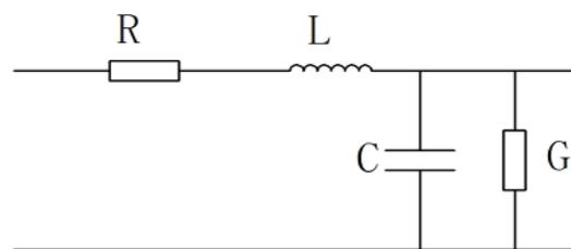
According to the transmission-line model, the impedance model of the TDR measurement cable is:
