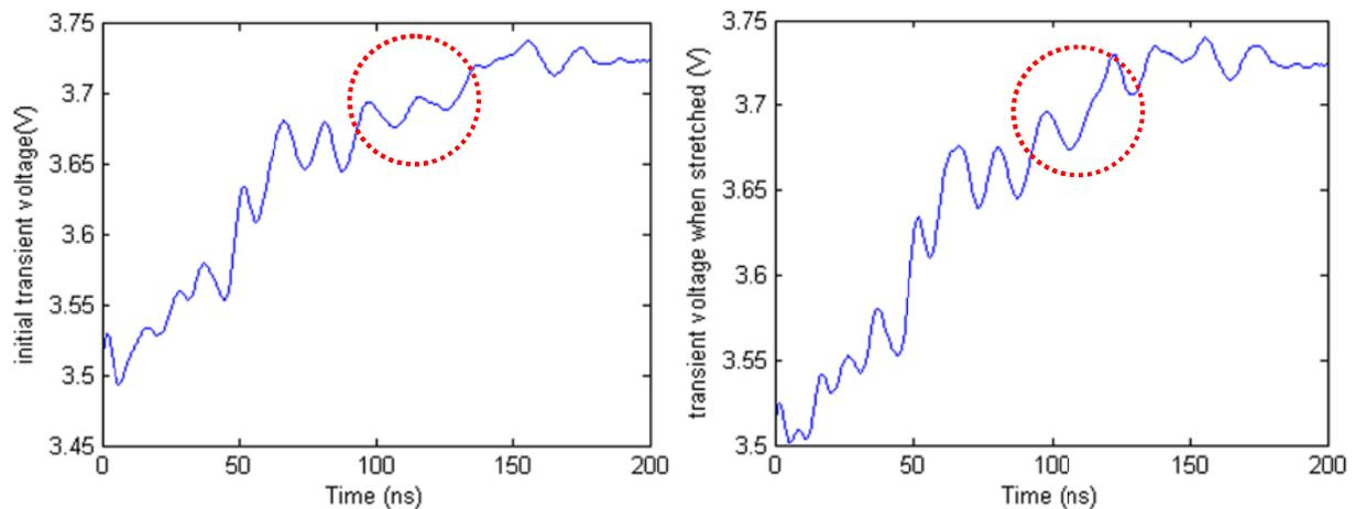
To obtain the local change of the transient voltage, a comparison method is applied in the TDR data processing. The difference waveform in Figure 17 is created by calculating the stretched waveform minus the initial state waveform. There is an obvious spike in the waveform which is caused by the stretching deformation. Besides the highest spike, there are many other lower spikes. Those spikes can be created by the TDR device measurement uncertainty.
