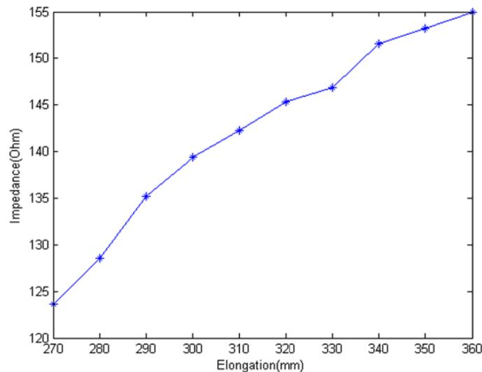
The experiment results verify our conclusion that the impedance of EHTSC increases when it is stretched. There is a difference between Figures 9 and 14. This difference may be caused by the connector and the non-uniform structure of the manual sensing cable.
