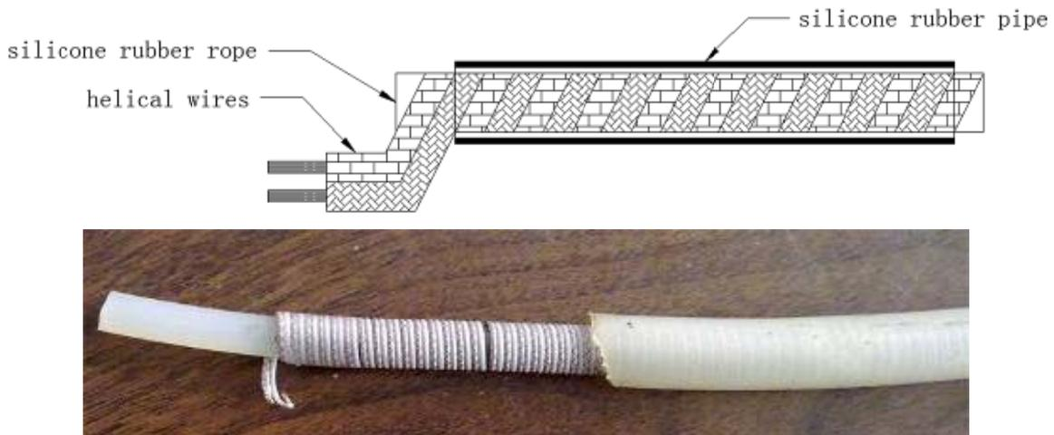
**Figure 5.** Parallel wires structure.
