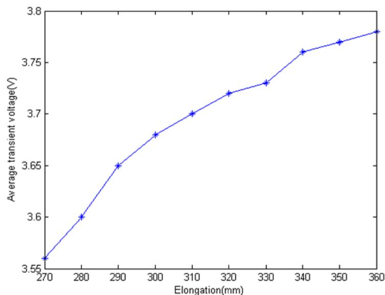
Figure 13 shows that the transient voltage  $U_C$  increases when EHTSC is stretched. And the rate decreases with the elongation increasing. According to Equation (8), we can calculate the impedance of EHTSC as Figure 14 shows.
