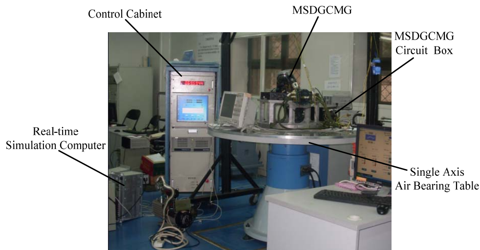
Figure 3. Experiment Scene of Semi-Physical Simulation.
