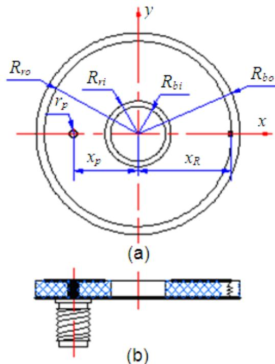
As a conventional annular ring patch antenna with parameter settings above mentioned, the outer radius of  $R_{bo}$  is at least 30 mm at resonant frequency of 2.4 GHz with very narrow bandwidth (as low as 1.7%). It is obvious that a conventional annular ring patch antenna is not suitable for the limited mounting space. As mentioned in Section 1, loading is an effective way to reduce antenna size. In this
