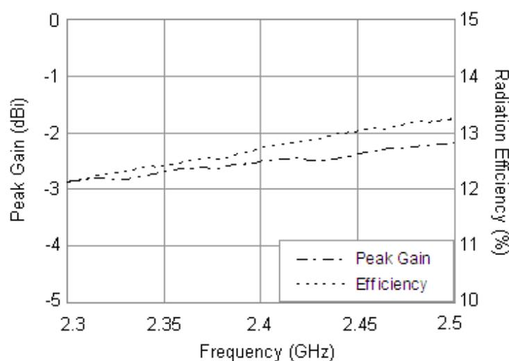
For further study to improve the gain of the antenna a substrate with relatively low permittivity can be used and its thickness increased suitably, however, the gain improvement may be relatively limited. Another approach to obtain an enhanced antenna gain is by covering the FR4 substrate with a high permittivity superstrate layer, and its thickness needs to be optimized to gain of the required
