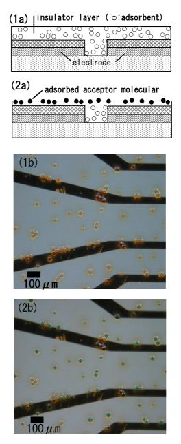
Figure 3 shows an optical microscope image of the inter-electrode spacing before and after adsorption treatment. Here, copper phthalocyanine was used as a dye for staining. After the adsorption of the dye and washing with distillated water all the  $SiO_2$  particles were stained a green color (Figure 3(2b)), whereas the color was transparent before the adsorption of the dye (Figure 3(1b)).
