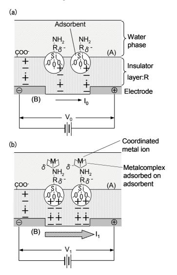
Figure 1. Schematic of an electrode chip and the detection mechanism of chemisorbed species.
