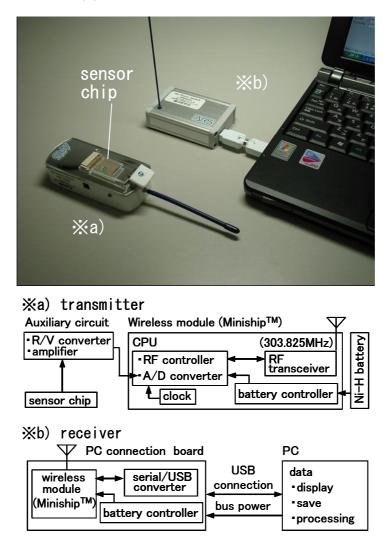
The developed wireless system in a package module "Miniship<sup>TM</sup>" was incorporated into both the transmitter and the receiver (Figure 4(a,b)). The device, which has dimensions of  $25 \times 25 \times 10$  mm and a weight of 7 g includes a PIC-type CPU. The power needed to drive this device (3.7 V) is supplied by a Ni-H rechargeable battery fitted within the transmitter and/or attached via USB to a PC. The performance of the device has been reported previously [10,11].
