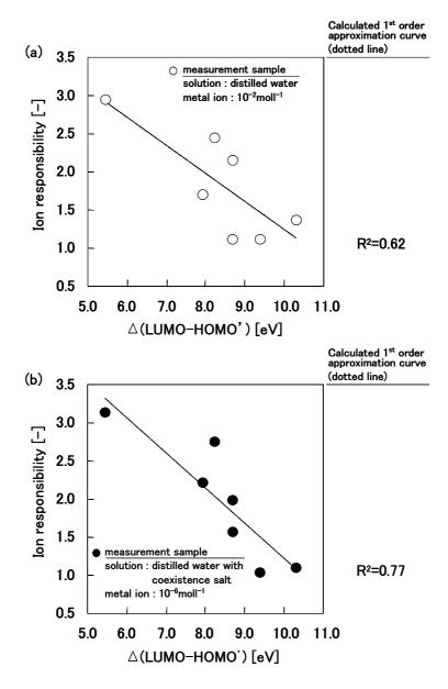
Figure 7(b) shows the ion response of each of the chelate molecules when the measurement sample solution contained  $10^{-6}$  mol·L<sup>-1</sup> metal ions. The actual measurement value of the ion response decreased with an increase in the  $\Delta$ (LUMO-HOMO') value with a 1st order approximation curve of 0.77.
