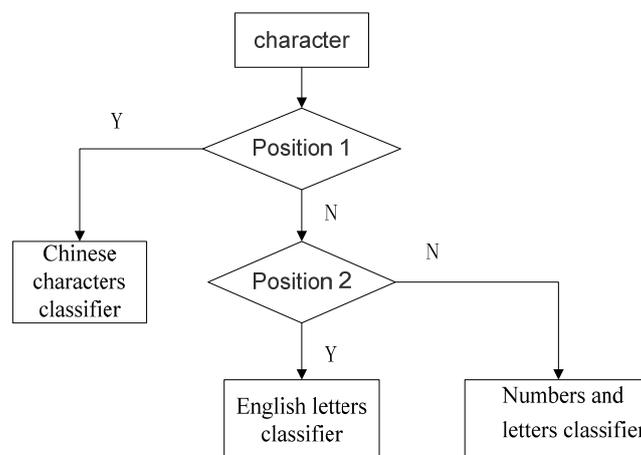
Firstly, according to the position, each character is categorized by the different classifiers, shown in Figure 18. Secondly, the characters that are to be identified with template characters are compared and their matching degree is calculated by the following equation:
