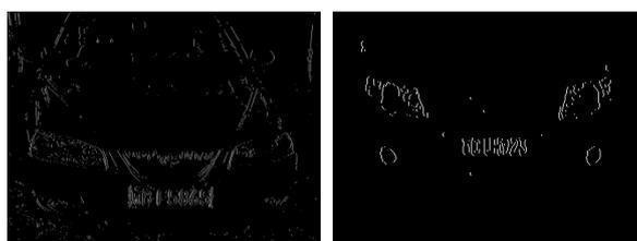
The first step of approximate localization is to detect the column range of the license plate. The whole image is scanned. Then the number of edge points, the number of jump points and the ratio which is between the number of edge points and the length of license plate area are calculated. If the column range meets the numerical interval changes range, this line and the starting point are marked, then repeating this process.
