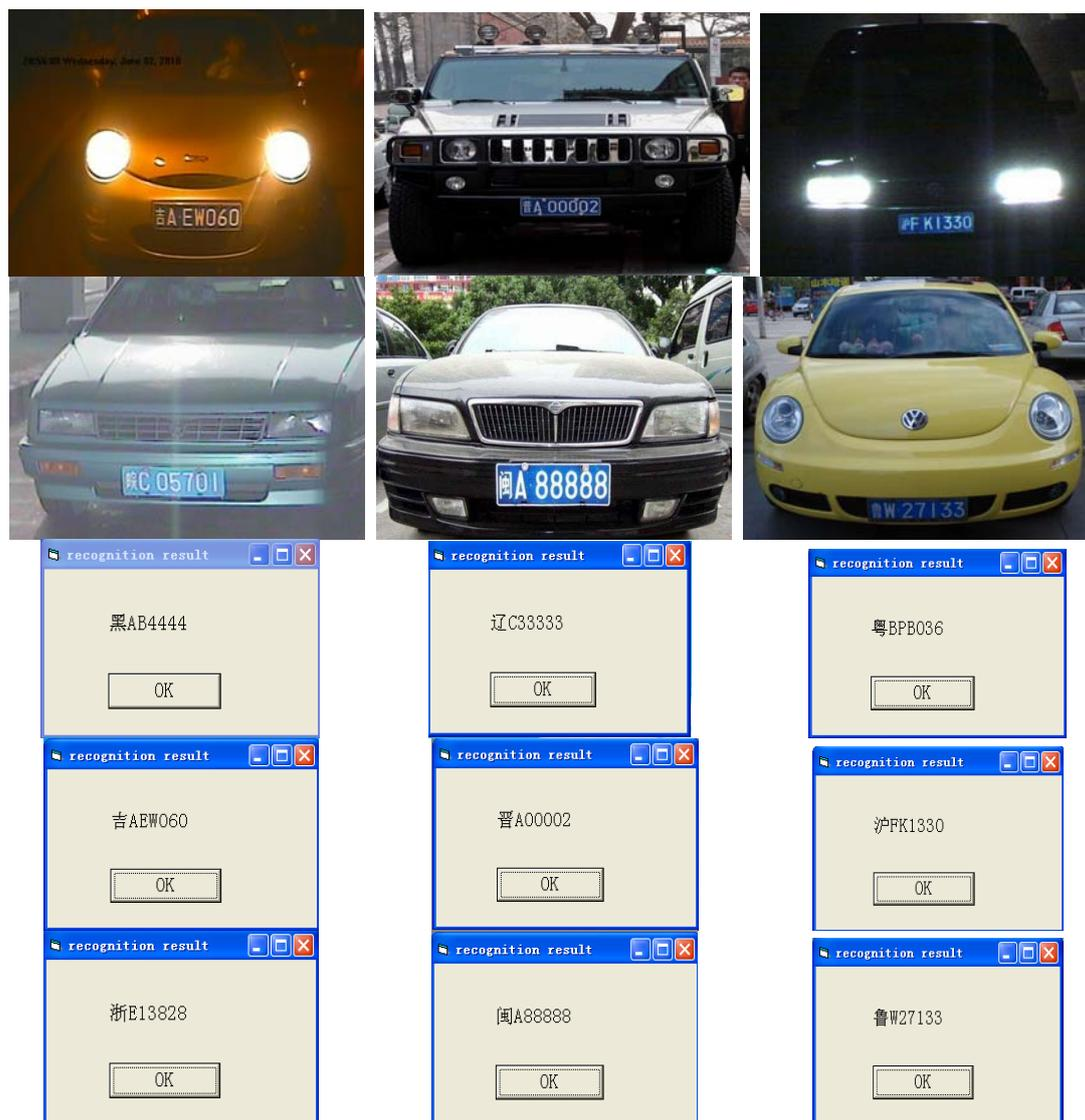
A total of 300 vehicles images obtained from community entrance gates have been tested. The recognition algorithm shows a high accuracy rate of 92%. We can conclude that the license plate recognition algorithm proposed here is capable of identifying passenger car license plates against complex backgrounds.
