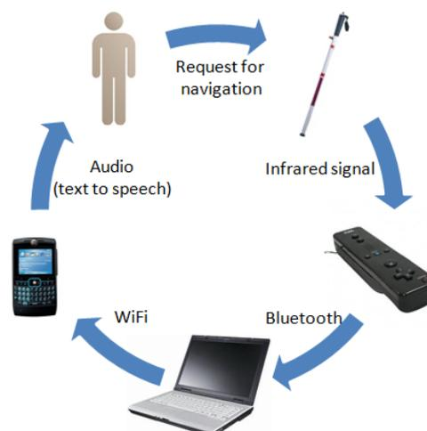
When the users request navigation information, they push a button on the cane. It activates the infrared LEDs embedded in the cane. The software application instantly tries to determine the user’s position and the presence of obstacles in the surrounding area. The user’s position and movement are
