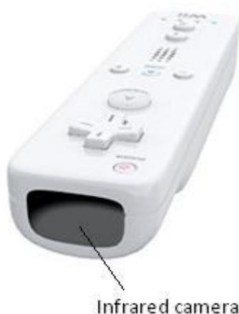
The Wiimote calculates the relative position of the light source. Therefore, by setting up the Wiimote in an indoor space, and knowing the exact position of the control, we can identify the position of any other object emitting infrared light in that area.
