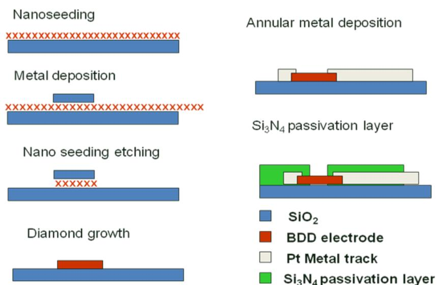
Several UMEAs with diameters varying from 2  $\mu\text{m}$  to 25  $\mu\text{m}$  have been fabricated using this technique. Most of these electrodes exhibited typical BDD responses. The complete EC characterization of one such UMEA (with 14  $\mu\text{m}$  diameter) is discussed in detail.
