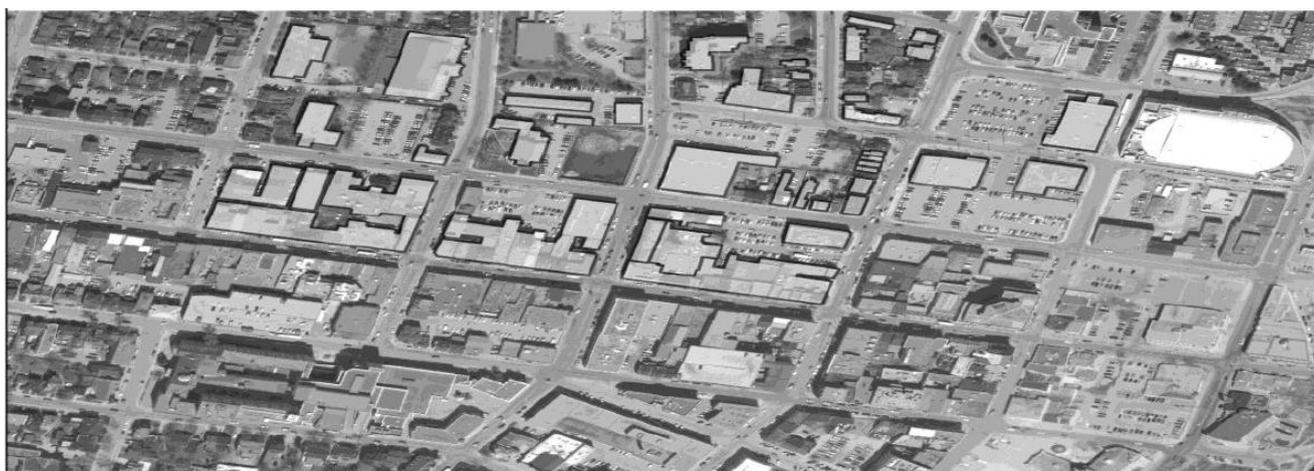
Among multiple levels of returns that LiDAR offers, the last returns of this area were used for roof construction since they were considered to most likely reach the closest to the ground hence the last object on the ground or the ground itself would be picked up by the last pulses [62,63]. Especially for buildings last and first returns are the same (in z values), which was checked with the current dataset.
