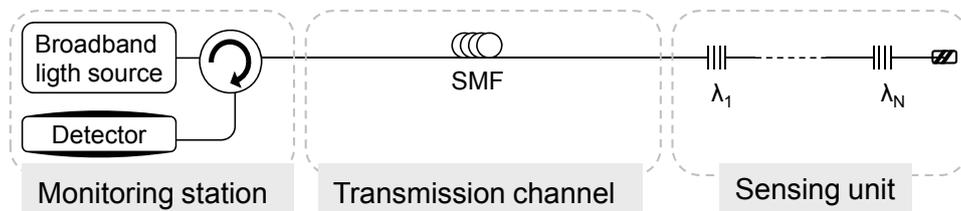
Nakajima *et al.* [40] introduced, for the first time, distributed Raman amplification into the simplest conventional FBG sensor system which is composed by a broadband light source, optical circulator, FBGs multiplexed in series and a detector. Figure 3 depicted the used scheme. The limited transmission distance of the conventional systems was overcome and the new system achieved to interrogate a FBG as far as 50 km with a SNR of 15 dB.
