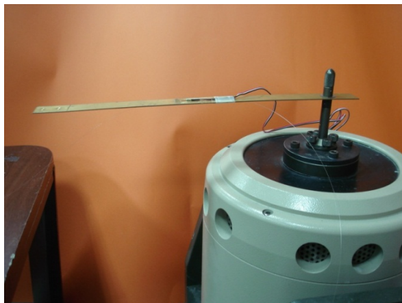
Figure 6. Cantilever beam mounted on a shaker.
