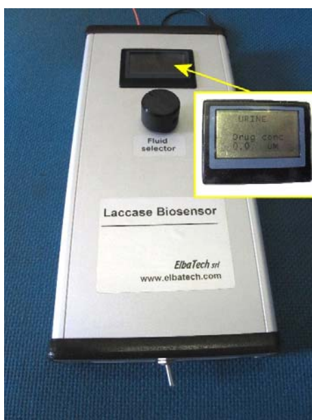
Figure 9. Prototype of laccase sensor jointly constructed with Elbatech Srl, Marciana (LI), Italy, compact and portable for all fluids indicated in Table 3.
