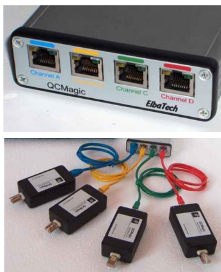
Figure 2. Nanogravimetric base-unit, able to drive up to four oscillating units ( Upper ). Oscillators unit connected via Ethernet cable to the base unit ( Lower ).
