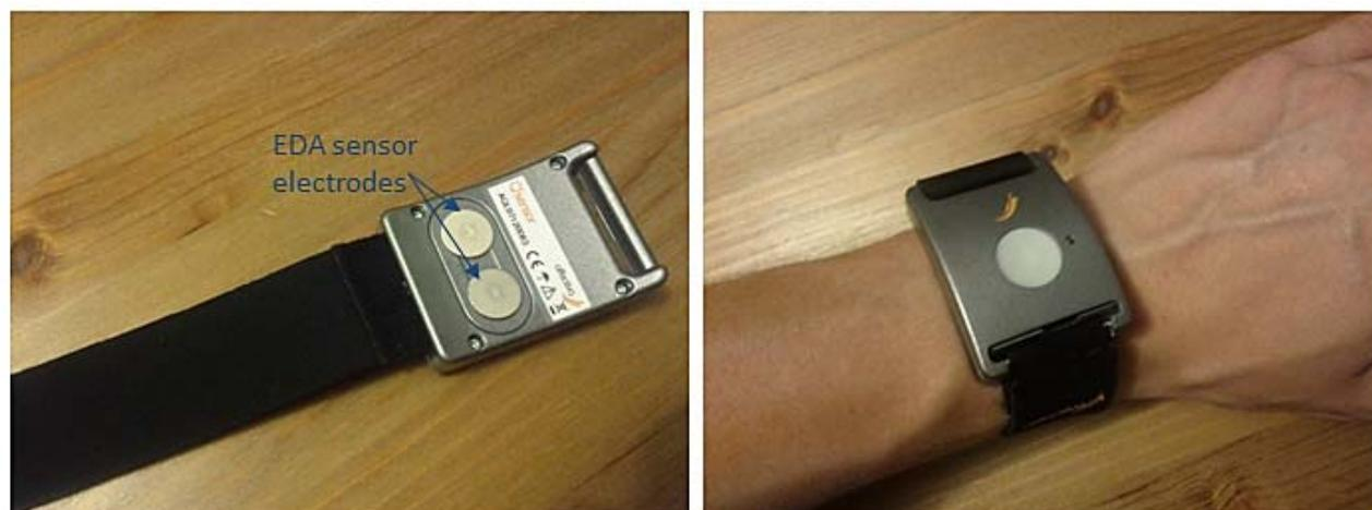
The signals acquired by EDA sensors are often corrupted by the users' movements during the measurement which is called motion artifact. Results can also be distorted by the users' physical
