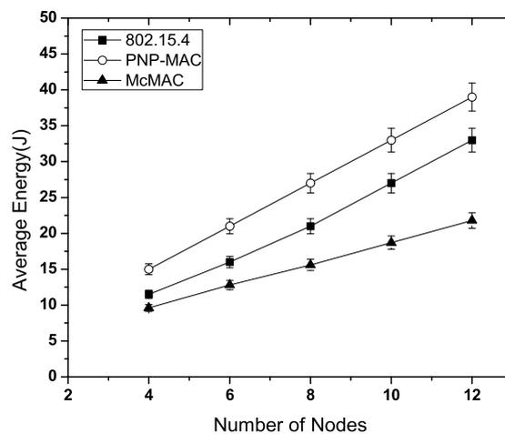
**Figure 12.** Average energy consumption of diverse periodic traffic at varying network size.
