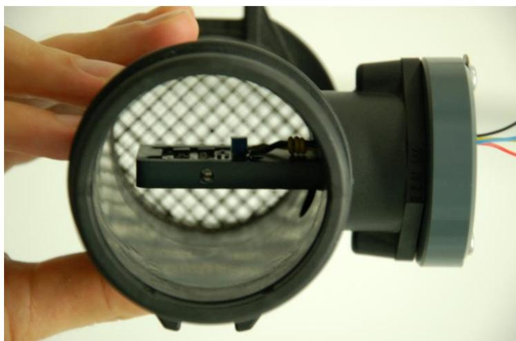
The fact that the flow channel dimensions of the second housing designed for the automobile engine are identical to those of the laboratory prototype allows for an estimated extrapolation of the results of Figure 6 in the case of air flow through the engine inlet flow tube. The amount of air flowing in the
