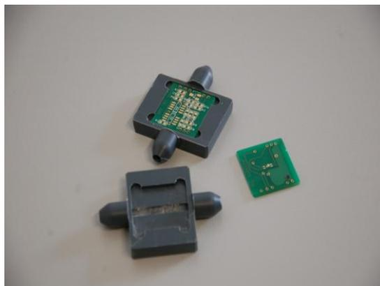
**Figure 5.** Picture of the full meter comprising the housing and the PCB with the electronics and the sensor on it mounted on the housing.
