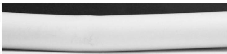
**Figure A8.** Curvature diagram of a pipe with curvature defect.
