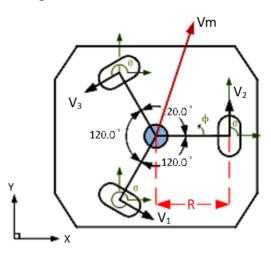
Figure 5. Configuration of the omni-directional mobile robot.
