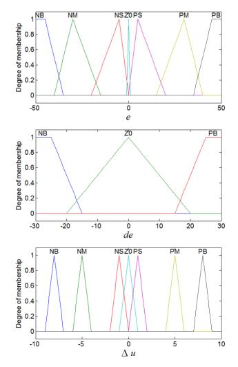
By developing rules of thumb based upon several measurements, premise and consequence are deduced and the tuned ranges of membership functions are determined accordingly. The rule base consisting of 21 rules for motor encoder compensation is given in Table 1, and an example is illustrated by:
