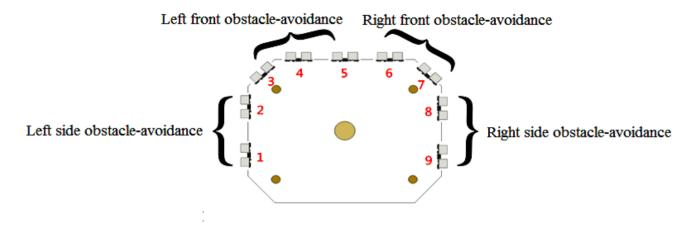
Figure 11. Ultrasonic distance sensors shown on the robot periphery.
