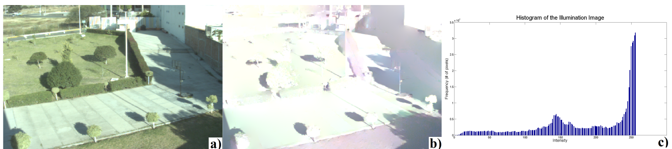
Figure 3. Example of an illumination histogram. (a) Input image; (b) illumination component computed with the method proposed by Matsushita et al. ; (c) Corresponding histogram of the illumination with two Gaussian tendencies. The highest Gaussian tendency corresponds to non-shadow pixels.
