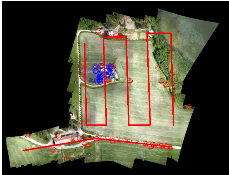
Figure 2. Flight routes of the reduced image block that was used in the SOCET SET processing. GCPs are in red and checkpoints are in blue.
