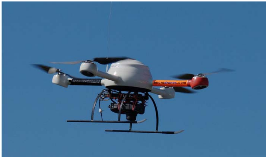
Figure 1. Microdrone md4-200 with a Ricoh GR3 compact camera.
