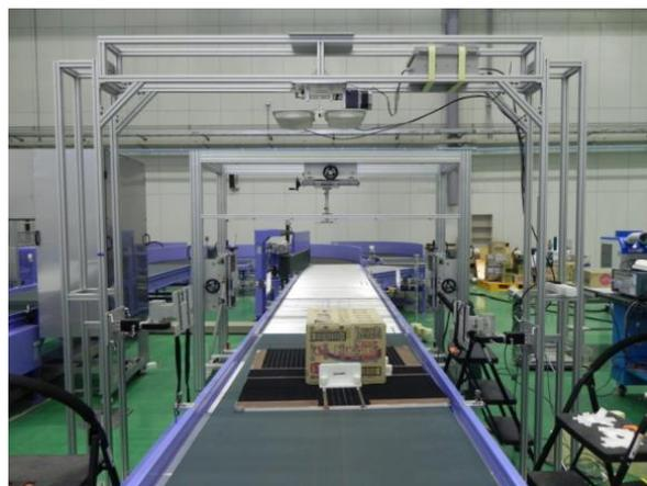
The experimental setup parameters are listed in Table 1. We have conducted two types of experiment with the conveyor belt gate system: employing an antenna control unit, and two arrayed fixed antennas. Linear and circularly polarized wave antennas were used for the experiments. For both the antenna control unit and fixed antenna experiments, we utilized two antennas using circular and linear type antennas.
