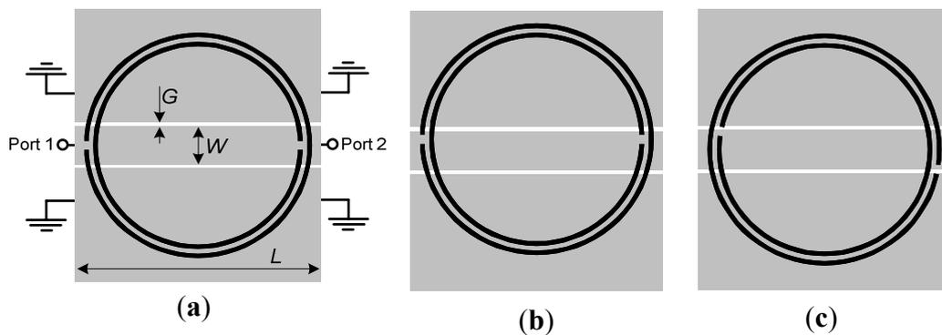
Alternatively, the fact that the SRR is not excited if the slits are perfectly aligned with the symmetry plane of the CPW can be explained since the symmetry plane of the SRR is an electric wall at resonance [5], *i.e.*, the distribution of charges is anti-symmetric with respect to that plane. However, the symmetry plane of a CPW structure is a magnetic wall for the fundamental (even) mode. Thus, the SRR cannot be excited if both symmetry planes (that of the CPW and that of the SRR) coincide.
