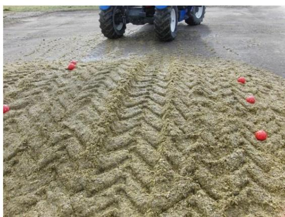
A network consisting of 15 sensor units was placed in a horizontal grid configuration at a distance of 0.10 m from the top of the silage stack (Figure 5). Measurement locations relatively close to the surface were selected because spoilage caused by the silage being exposed to air is initiated at near surface locations.
