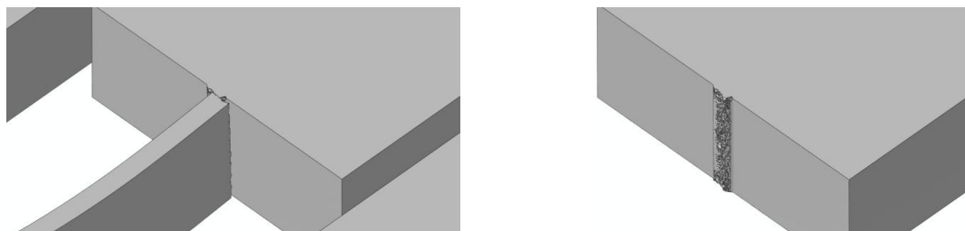
Figure 14. Failure mechanism induced by the tension-dominated loading (side-B drop).
