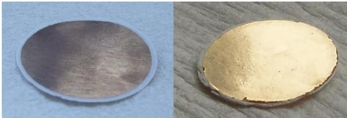
**Figure 6.** Scanning electron microscopic (SEM) images of the gold layers on mesoporous silica pellets; the layers have a thickness of 10 nm (left) and 50 nm (right), respectively.
