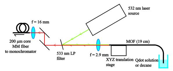
Figure 3. Experimental configuration for fiber-based fluorescence measurements.
