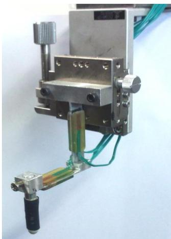
**Figure 4.** Photograph of experimental apparatus for MR haptic display.
