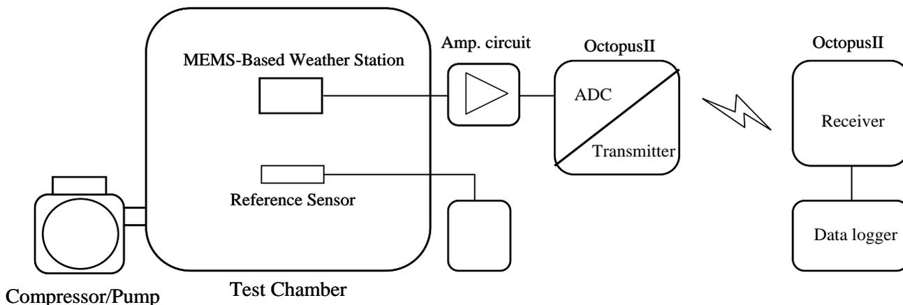
The electrical signals associated with temperature, humidity, pressure, airflow velocity and changes in direction were amplified and converted into signals of a specific voltage using an analog circuit, connected between the sensor array and the Octopus II sensor node. Through the Octopus II sensor node, the analog voltage signals were converted into digital signals and transmitted wirelessly to the data logger.
